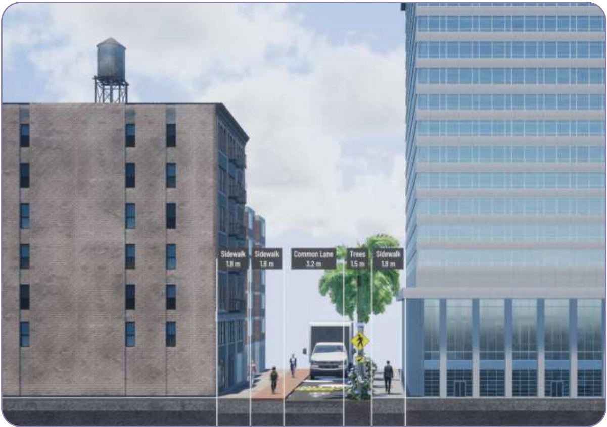
Figure 24: Final Cross-Section Note: Author's own work
